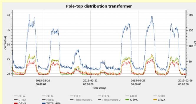
**Figure 3: Profiling a distribution transformer - Estimating kVA for phases A, B, C and total**
